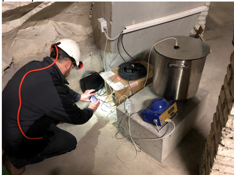
Fig.2. Installation of Rotaphone station RICC inside the repository of nuclear waste in mine Richard near Litoměřice
