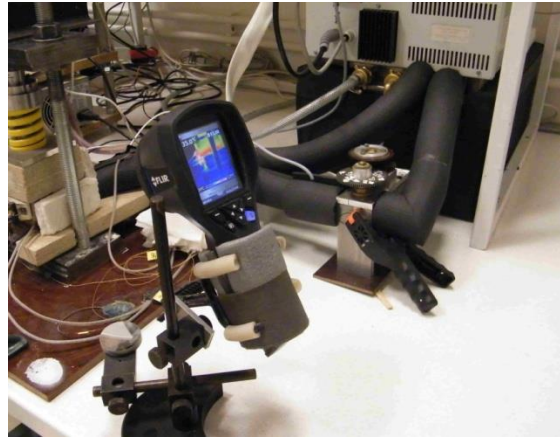
Fig. 24-3. Automated characterization equipment for testing of thermoelectric modules and materials.
