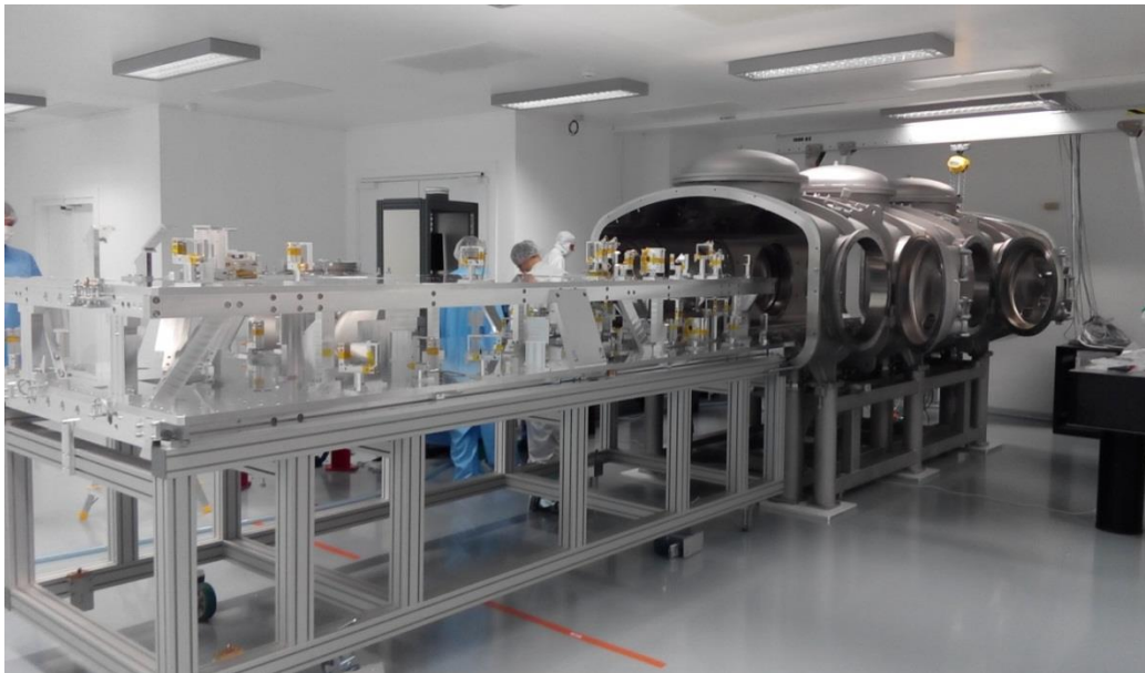
Assembling the ps vacuum compressor for the L1 laser of ELI-Beamlines, designed by the Dept 91 research and technical team, in cooperation with the engineering support by Dept. 93.
