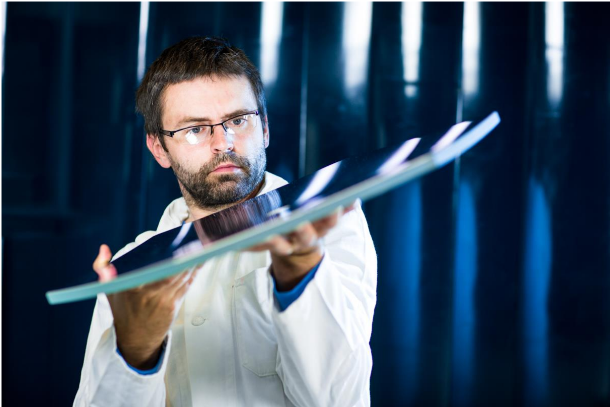
Figure 5: L. Nožka examines one of the mirror segments produced for the fluorescence telescope at the Pierre Auger Observatory. |
